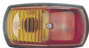
Part # NA85760 Side Marker Lamp (Red/ Amber)
