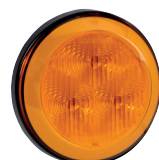
Part # NA94300 9-33 Volt L.E.D Rear Direction Indicator Lamp (Amber) with 0.5m Hard-Wired Sheathed Cable and Black Base
